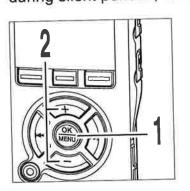
While the recorder is stopped or during recording, press the **MENU** button for 1 second or longer.
